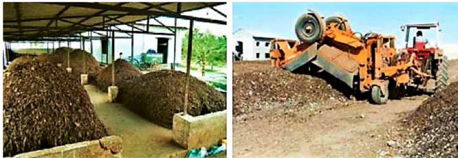
Windrows which have been turned manually (left) and mechanically windrow turning (right)
