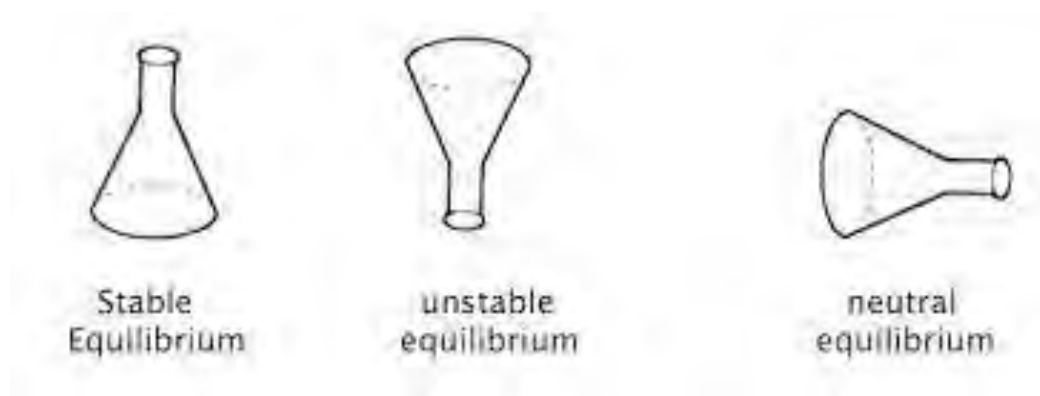
Fig 7.13; Showing the equilibrium condition
