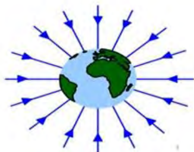
Fig7.4: Gravitational field strength is the force per unit test mass
