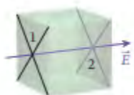
Fig 20.13: Imaginary empty box in a uniform electric field.
