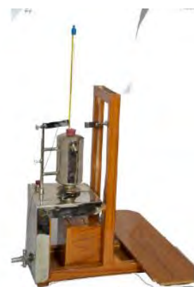
[Fig. 11.3: Determination of specific heat capacity of a solid from the method of mixture]
